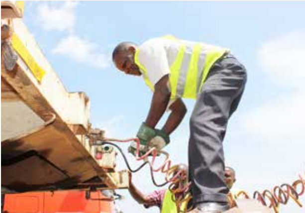
Opoka coupling up the Suzie's/ air & electrical lines
